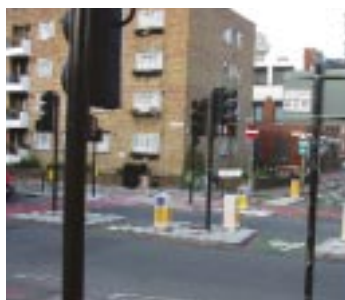
Parallel crossing provides for direct routes for pedestrians and cyclists
