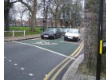
Centrally located ASL lead-in cycle lane is useful when there is a left-turn-only traffic lane
